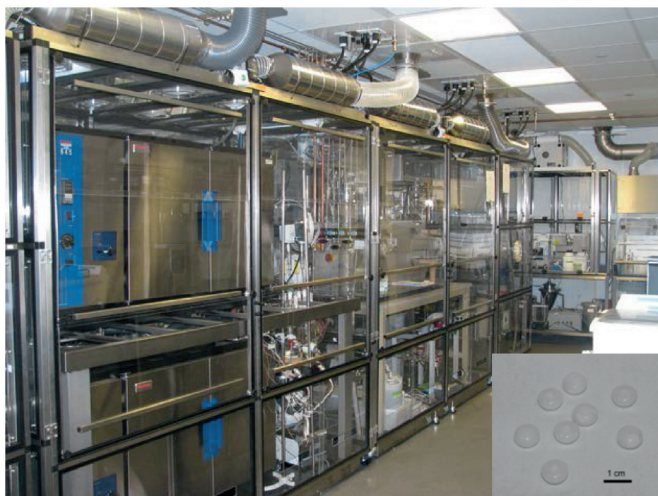
Scheme 61. End-to-end, integrated continuous manufacturing plant for the synthesis of Aliskiren. The inset shows the formulated tablets. Image adapted from Ref. [8a] with permission. Copyright 2013, Wiley-VCH.
